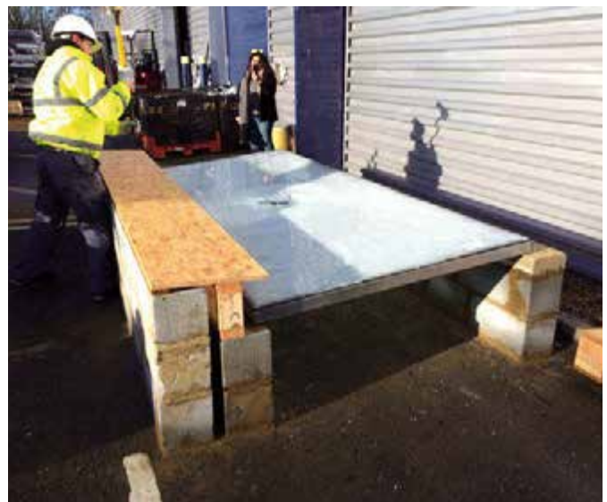
The witnessed testing of a sample glazing panel, made to match exactly the new glazing to go over the East Terrace stairs
