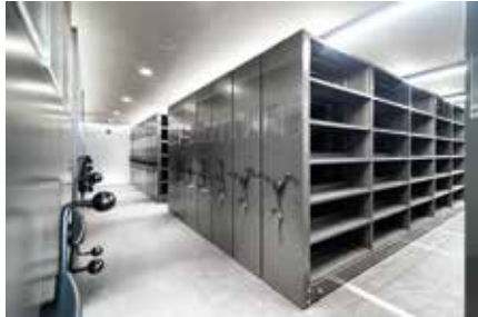
The Library Extension is much larger underground on plan than the offices above, and the moveable book stacks allow for high density storage.
