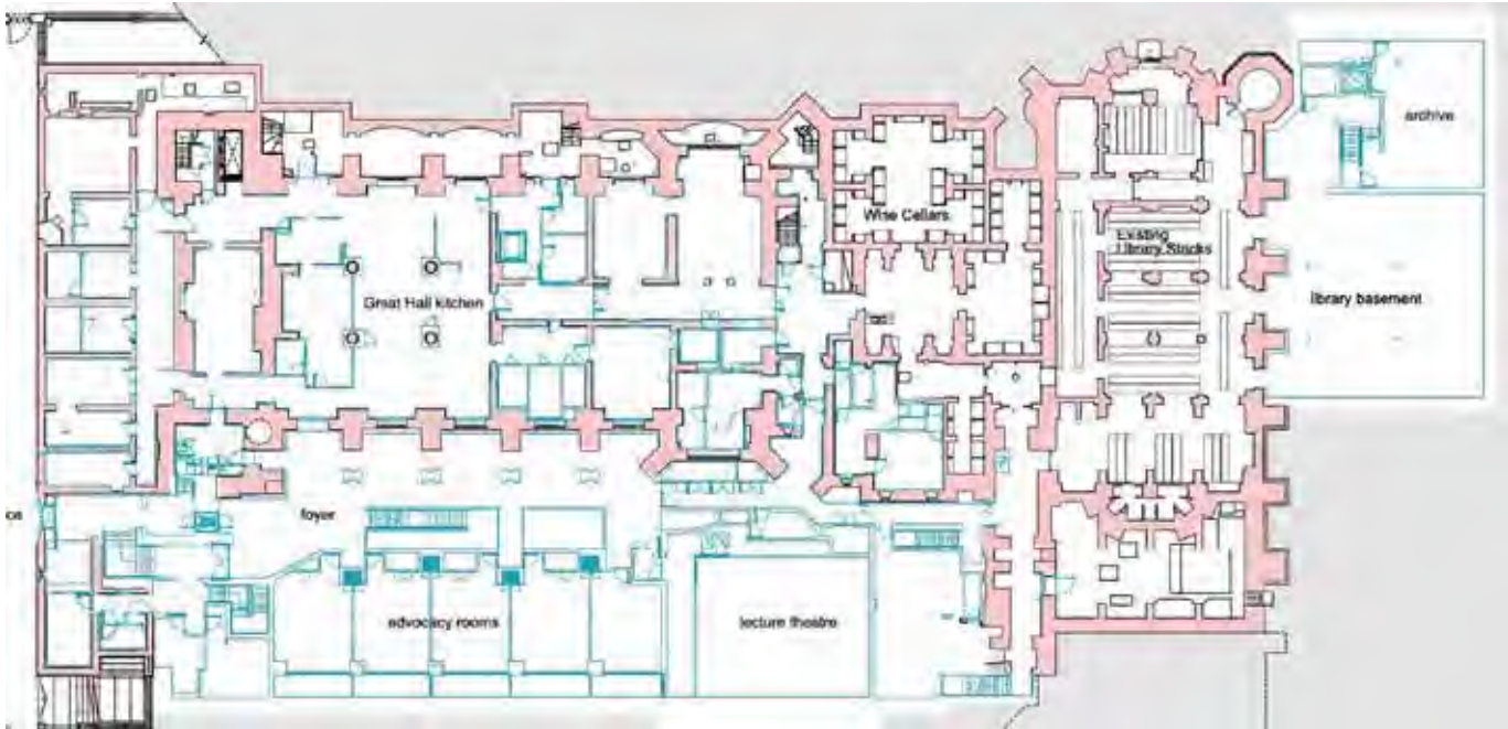
Basement plan showing East Terrace Extension at the bottom, North Library Extension on the right and works to existing Great Hall building in the centre
